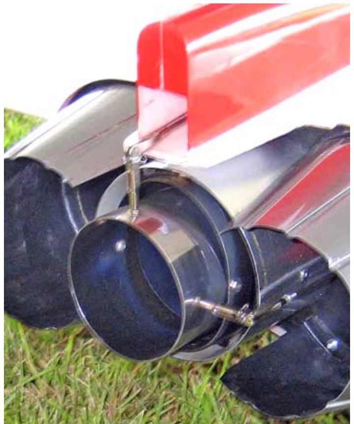
Thrust vector control setup in "neutral."
