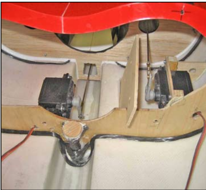
"Rudder" and "elevator" vector control servos installed near the tail pipe. A baffle and lots of heat shielding (added later) protect the servos and leads.
