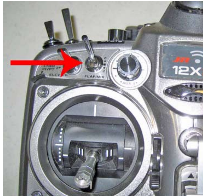
Since the Eurosport has no flaps, the flap/mix switch (arrow) is a convenient location to select "flight modes" (same as "flight conditions" for Futaba users).
