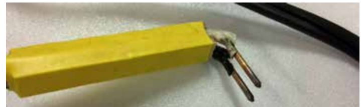
Close-up of the home-made electrodes from household wiring.
