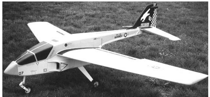
Ray Davis, JPO District I Rep, flew his modified, swept wing Facet 1200, powered by a Wren MW 44 Gold turbine. At just 10 pounds, it is a real performer.
