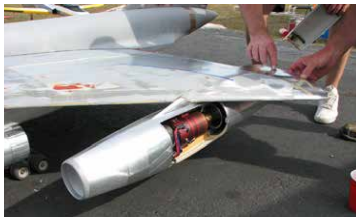
A closeup of the number one nacelle on the B-58, with KingTech K-60 installed.
