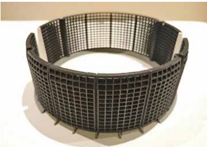
The Cascades (side thrust reverser) assembly.
