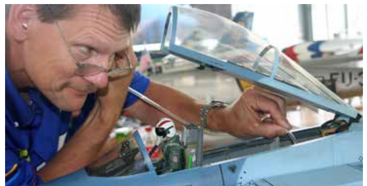
"Doc" Harris using his stethoscope-tubing skills to help Jason find an air leak in his retracts system.
