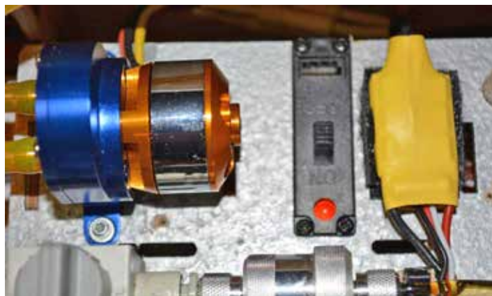
Pump, speed control, and switch installed on tray.
