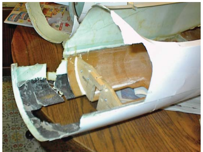
Fuselage damage. Note missing carbon fiber in front of nose wheel opening
