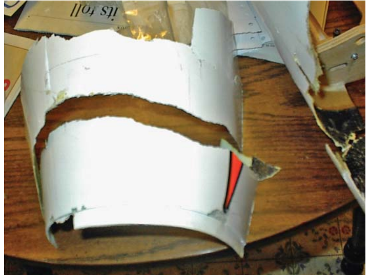
Broken upper Fuselage with missing flange pieces, the flange pieces were repaired with a cured, flat fiberglass and epoxy layup fabricated on a glass shelf, and cut into strips used as a backing for additional cloth and resin buildup.
