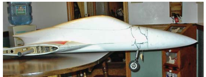
Repaired right fuselage side ready for sanding.
