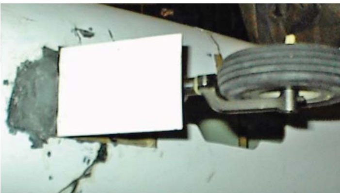
Repaired fuselage and carbon fiber fwd of nose gear using packing tape and a carbon fiber /epoxy resin layup.
