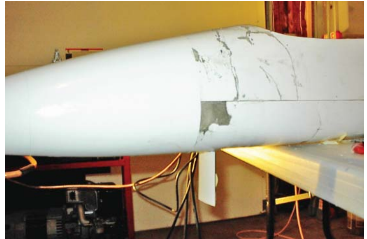
Repaired left fuselage side, note in-aircraft fabrication of missing piece (gray area) in the photo above.
