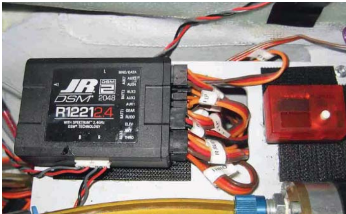
Same size 1221 Rx replaces old R955 perfectly. Note labels on servo leads and red Data Logger located to the right.
