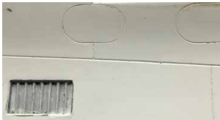
Rafale surface detail after stripping paint with SEM.
