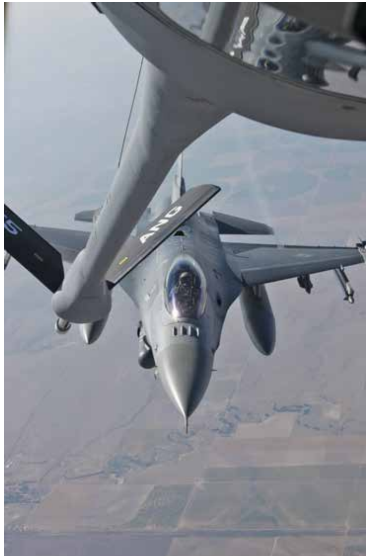
A pilot comes into the contact position so that the boomer can plug in and complete the fuel transfer.
