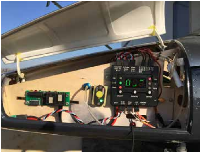
Global L-39 nose compartment & latches.
