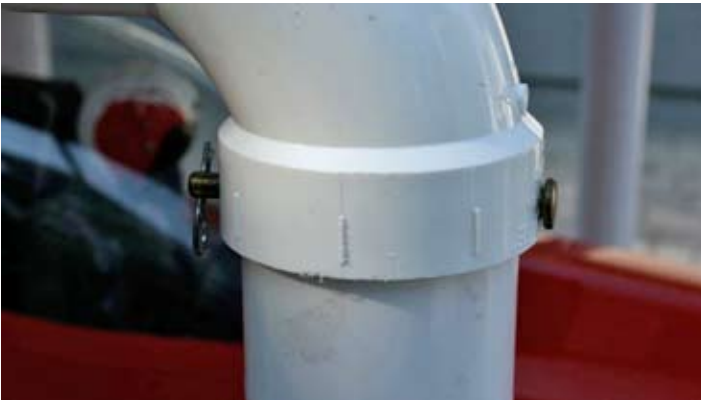
Removable pins hold the top tier in place, but make it easy to remove if you have a large tailplane model you want to carry on the middle rack.
