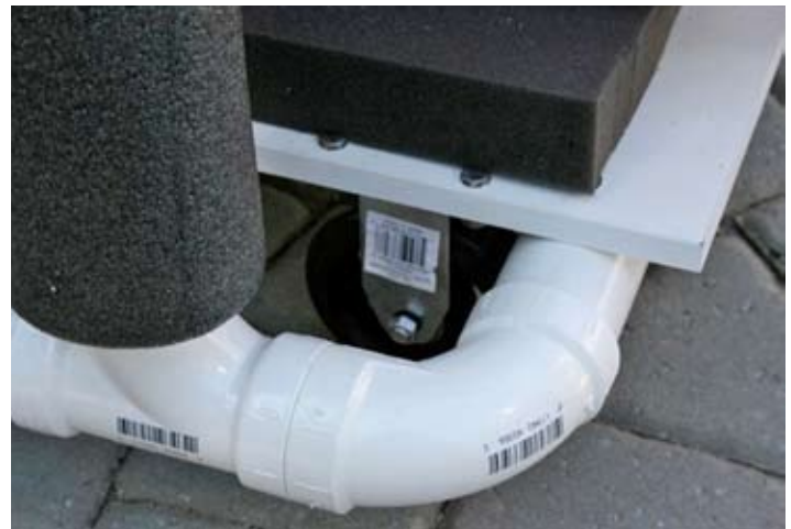
Four inch casters provide mobility. Two freewheeling casters up front make maneuvering easy.
