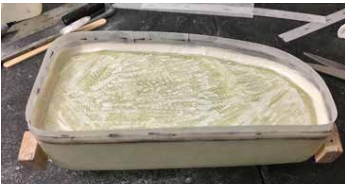
A 1/16" thick piece of G10 was Hysol'd into the tank to separate the fuel and smoke compartments. \frac{3}{4} " wide strips of 0.010" thick G10 were then glued \frac{3}{8} " inside of the tank (leaving \frac{3}{8} "-inch protruding past the edge).
