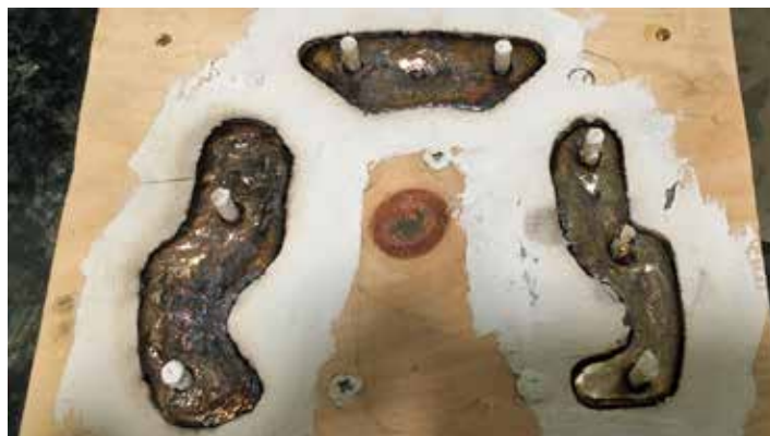
Three custom lead weights to fit in the irregular and narrow space between the engine and cowl in my Spitfire . The outside edge of the weights clears the cowl and the inside shape clears the DLE55 engine.
