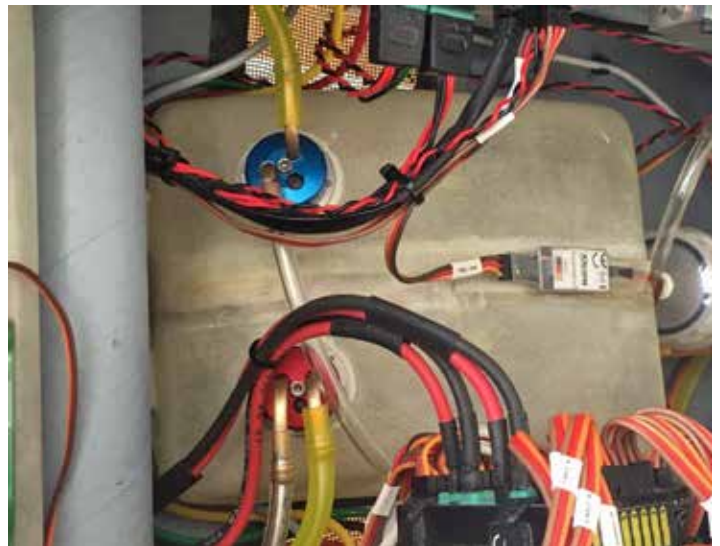
The completed "combi" tank is narrower and doesn't block the air inlets, yet provides an additional 24oz of fuel (12 minutes total) and 21oz of smoke fluid.
