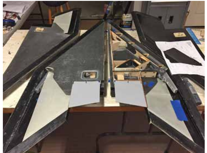
Inboard Wings, Lower Sides in the Molds.
