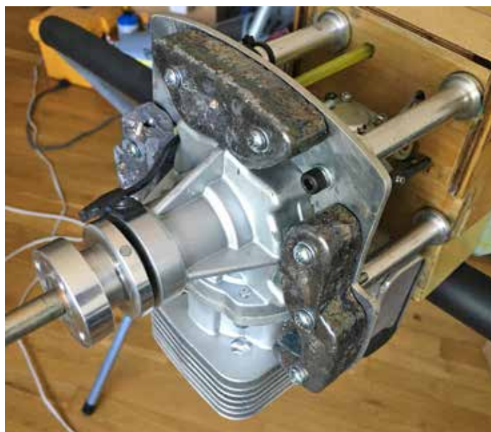
Weights installed on plate mounted in front of engine mounts. Weight at left side of photo was trimmed as needed to balance the plane.
