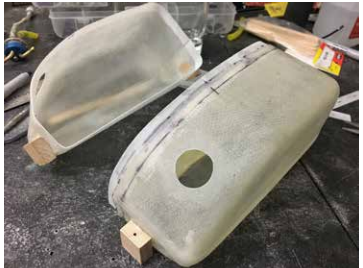
The G10 strips align the tank halves during reassembly and provides additional bonding surface and strength. After joining, \frac{3}{4} "-wide fiberglass cloth is then wrapped around the joint and glassed.
