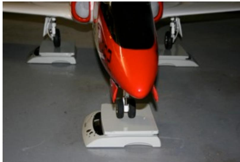
Place the plane on the scales, wheels centered, and record weights. If you are working with a tailwheel aircraft, block up the rear scale such that the plane is weighed in a level attitude.
