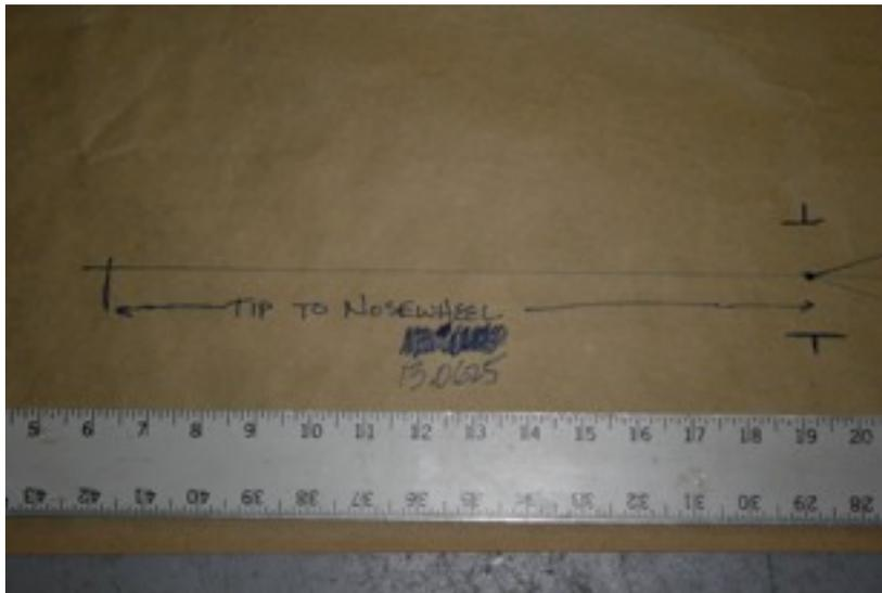
Next, capture the measure from the nose wheel to the main, and then from one main to the next. See photos at right
