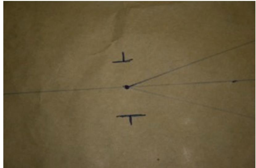
Remove the aircraft from the paper, and mark a dot at the exact center of each wheel, where the axel line would bisect the two wheel edge lines. Using a long straight edge, connect the three dots, forming a triangle. Also draw a line between the two marks you made to identify the leading edge.
