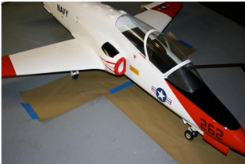
Using a large T Square, mark the position of the tip of the nose on the paper. Also, mark the both sides of each wheel and the axel point as shown in the following pictures. If you are doing this for a tailwheel aircraft, make sure the plane is in a level flight position, that is, with a wing incidence of zero. This will require that you block up the aft end of the aircraft.
