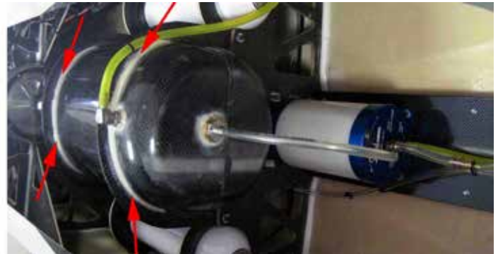
6.5L fuel tank and large air tanks are secured with laminated brackets. Fuel tank brackets need to be trimmed to fit and glued securely to the tank (red arrows). Brackets are held in place with 4/40 bolts and blind nuts.
