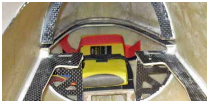
Battery tray with receiver A123 batteries (left). Battery slides into slots and secured with two 4/40 bolts and blind nuts (right). I located the ECU battery underneath.
