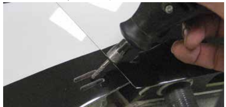
Slots for control horns are pre-cut on all control surfaces but need to be enlarged and deepened to fit the horns.
