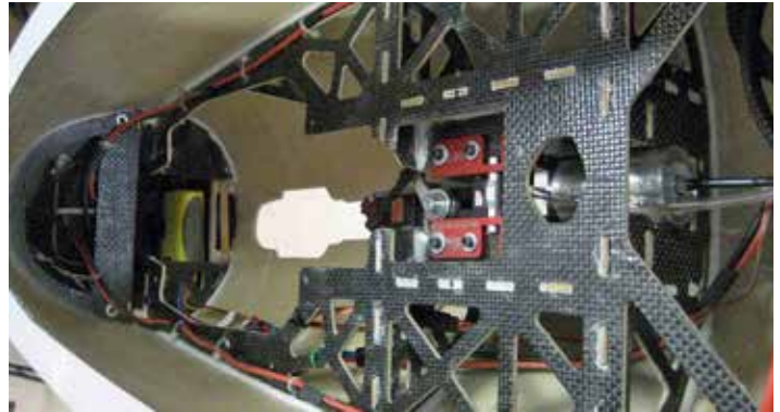
View of nose gear mount structure and battery tray installed forward. Main component tray is 12" X 10.5." I fabricated a second tray, (bottom left) so I could locate the UAT and ECU closer to the fuel tank and turbine. JMP hi-flow fittings throughout.
