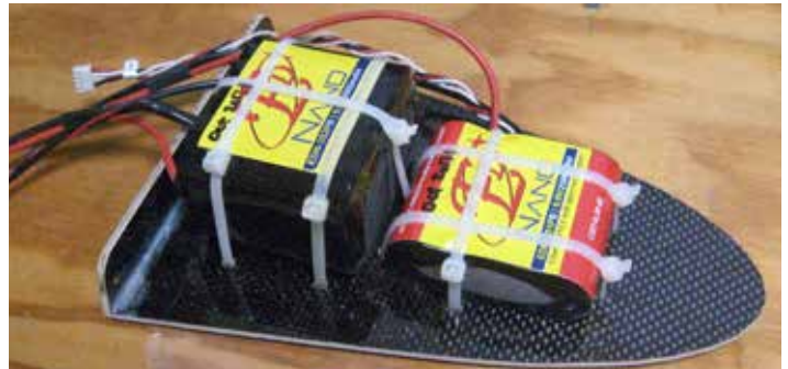
Battery tray with receiver A123 batteries (left). Battery slides into slots and secured with two 4/40 bolts and blind nuts (right). I located the ECU battery underneath.
