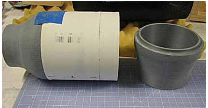
Gray parts shown to be epoxied to a PVC tube to make a plug shape, on which a fiberglass bypass will be laid up.
