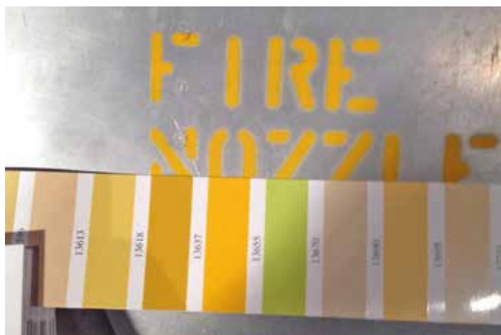
Comparing the color of markings to a Fed Std color fan deck. FS13655 paint.
