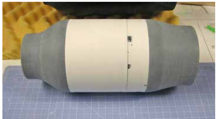
Gray printed parts epoxied in place to form the bypass plug shape.
