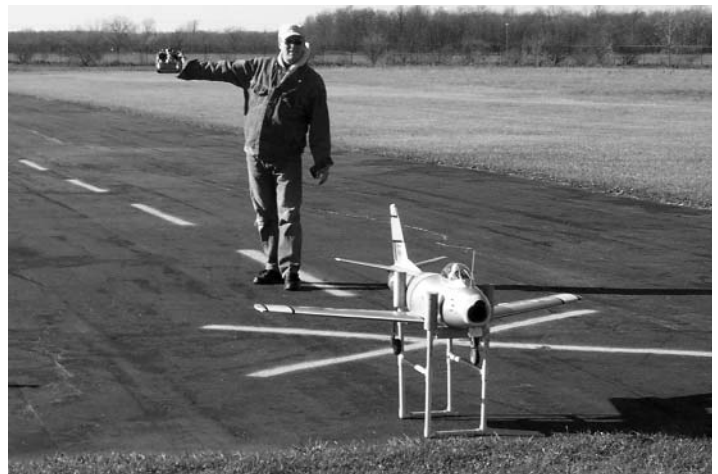
Photo Of F-86 On PVC Stand - Two Feet Above The Ground And Author Holding Tx For Test
