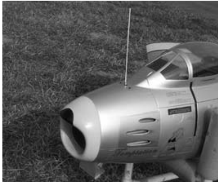
Photo Shows The Deans Mini Antenna Mounted On The Fuse
