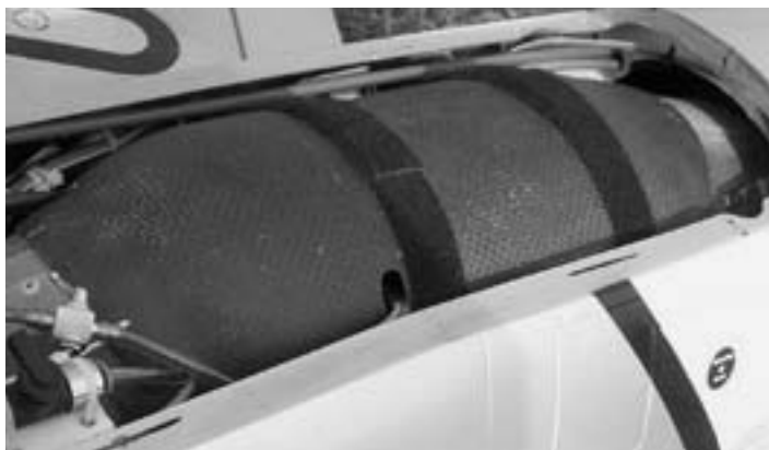
The Conventional Antenna Can Be Seen Routed In The Tube, Alongside The Shroud At The Top Of The Photo
