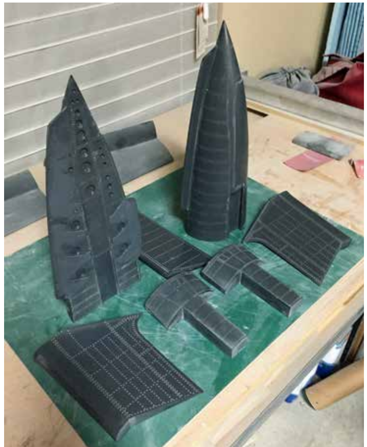
Detailed plug parts ready for molding.
