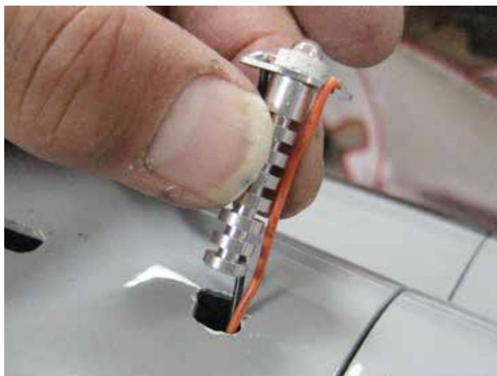
Fuselage red beacon strobe. Cutout just large enough for heat sink and wires.
