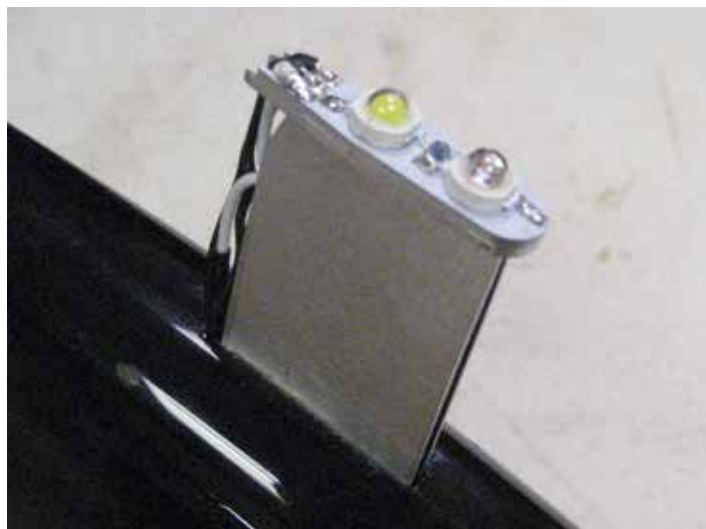
Wingtip nav/strobe unit. Glued in place with black silicone.
