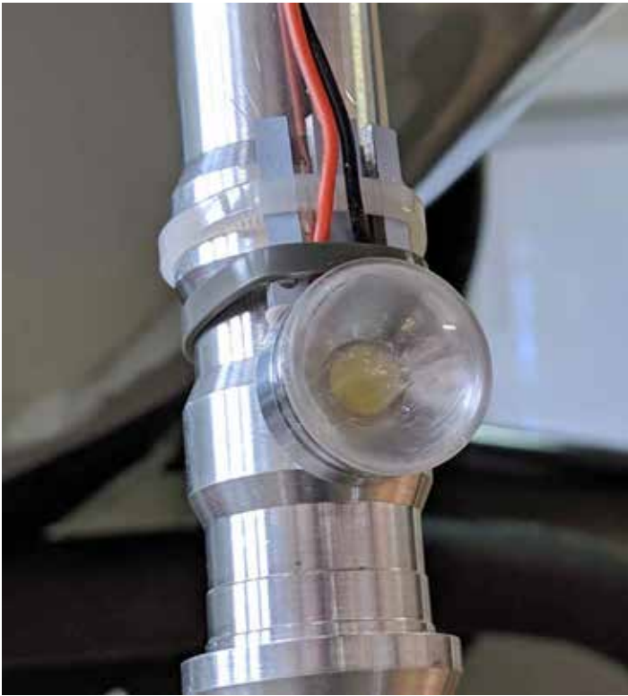
Nose gear landing light. Secured to strut with cable ties around heat sink.
