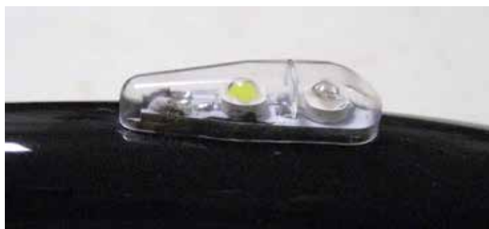
Finished wingtip unit. Clear lens held in place with a thin application of clear silicone.
