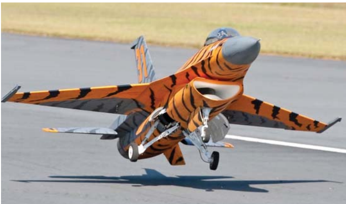
Skymaster F-16 flown by Ritchie Holt. The 30-pound jet is powered by a P-160.
