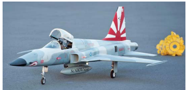
Incredibly detailed Fei Bao F-5 by Jed Jacobsen. Features lights, drag chute and a fully-functional, scale canopy-opening mechanism designed by Jed.
