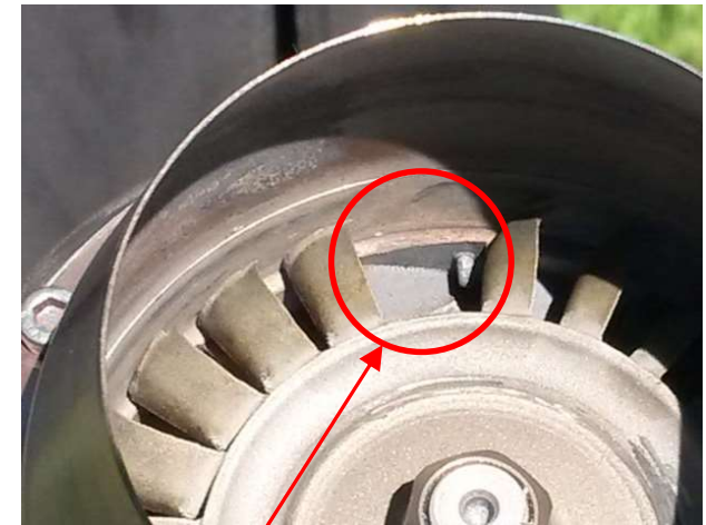
Missing turbine blade
