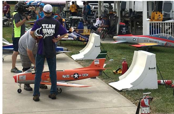
Typical startup area. Note: blast defectors, fire extinguishers, people are forward of turbine, pilot and spotter are both are physically restraining the plane from moving.
