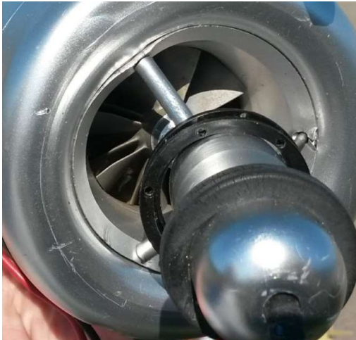
Crash Damage - Starter motor mount and inlet bent
