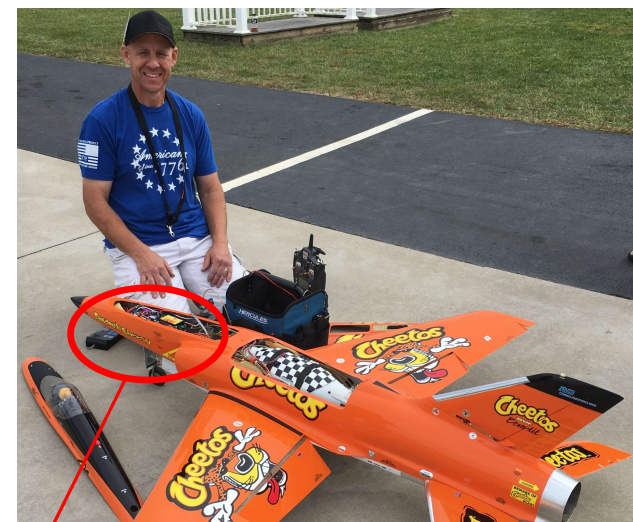
GSU connected to ECU before turbine start. This modeler cares about his turbine and his model (which are both over 10 years old).
