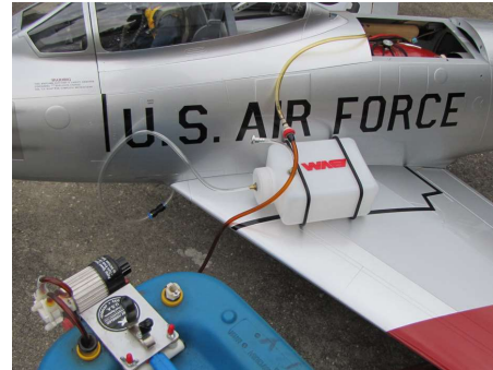
Fueling using a Jersey Modeler 5 gal electric fueler and overflow tank.
