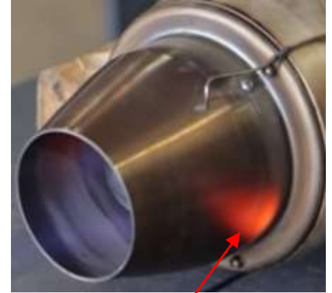
Hotspot on nozzle due to compressor damage (likely FOD or crash loading)
