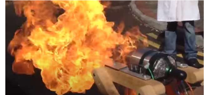
Turbine hot start on test bench
