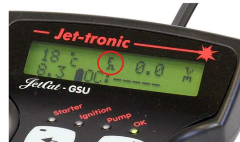
Jetcat GSU showing failsafe activated
