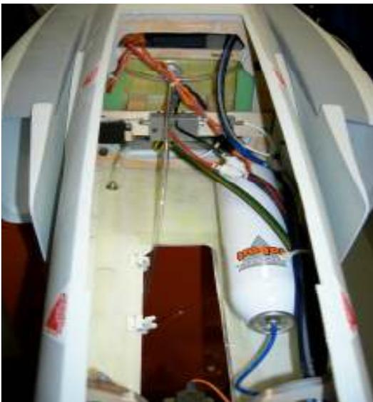
Center tank shown with ply brace, air and brake valves attached
