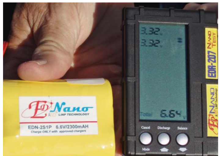
EDR-107 Tester displaying individual cell voltages on a 2-cell A-123 Receiver pack. Each cell is above 3.2V and it is safe to fly another flight before recharging. A test lead allows checking batteries through the charge port on a receiver switch.
