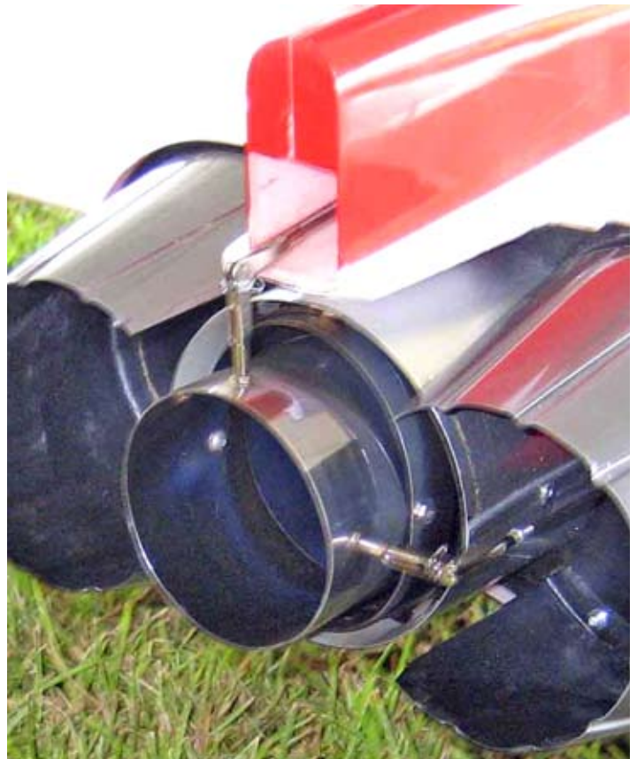
Thrust vector control setup in "neutral."
