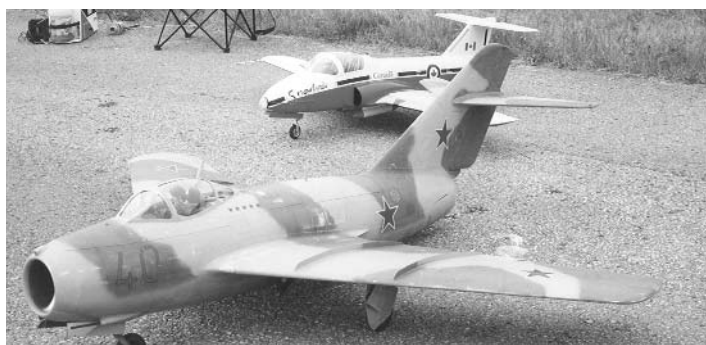
Marty Cowan from Belleville, Ontario flew a Comp-ARF MIG-15 with the new Wren Super Sport Turbine. This turbine gave the MIG sparkling performance even though it appeared lost in the belly of this jet. A scratch-built CT-114 Tutor jet is in the background.
