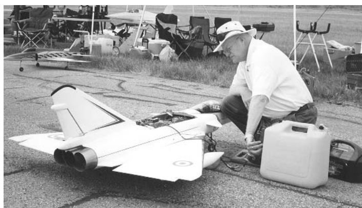
Gilles Pelletier fuels his Mirage 4000 for another successful flight at Quinte '05. This Mirage was originally built and flown with twin-ducted fans but is now turbine-powered by a single engine.
