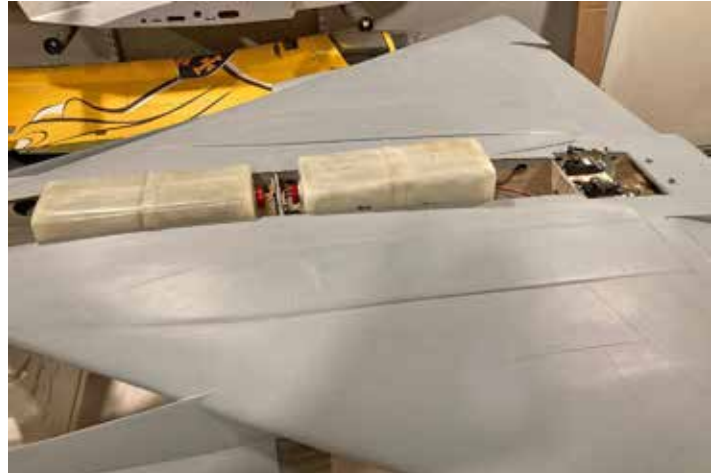
Hustler build: Fuel tanks, elevon servos and linkages installed.
