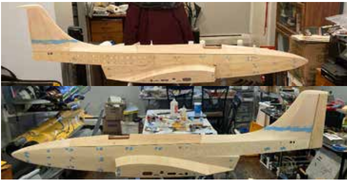
Glassing the fuselage is a lot simpler with the holes filled.
