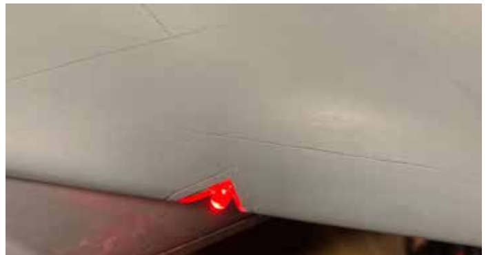
Light system installation in the wing. Now to mold the Lexan cover.
