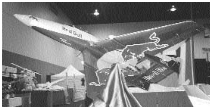
Terry Nitch's KingCat was flawlessly finished in the Red Bull color scheme and powered by an AMT AT-400 Auto-start turbine.
