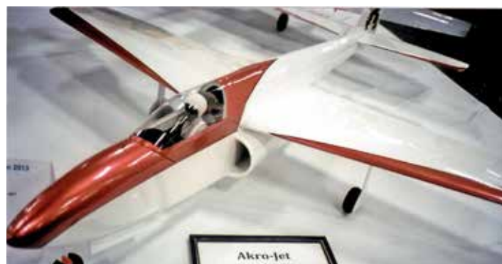
Keith Shaw, from Ann Arbor, MI scratch built, and took home First Place - Film Covering at Toledo. It is based on the Temco TT-1/Polish Iskra trainer jets. It is an edf-propelled by a Change Sun 90mm fan unit.
