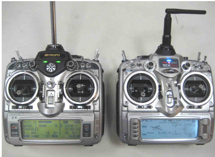
12x (right) is similar to 10X but uses buttons and rolling selector to enter data. Extra two Aux knobs are located on top.
