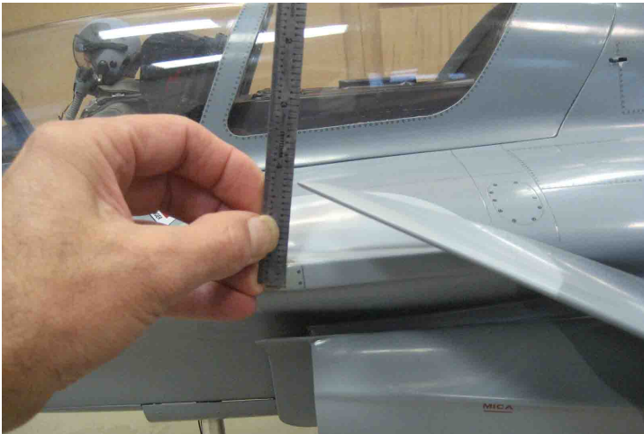
Check neutral position and measure throws for all control surfaces carefully before first flight.
