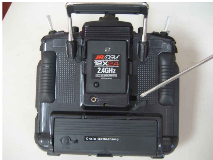
Phillips screwdriver points to friction access hole
