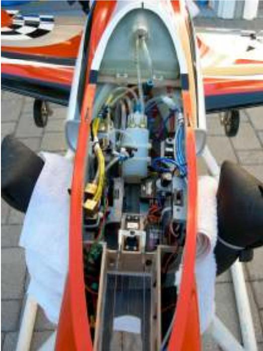
I also replaced the 10-ounce header tank with a BVM Ultimate Air Trap. The plywood structure that was designed for the header tank is easily modified to hold the UAT. Other than these minor points, the model building process conforms very well to the instruction manual.
