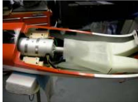
At just under four inches in diameter, the Falcon fit nicely into the bypass, with plenty of room for cool air to move around the engine. Since the turbine sits to the rear of the Center of Gravity, weight is also an important consideration. At 3.3 pounds, the Falcon is a solid choice in this regard.
