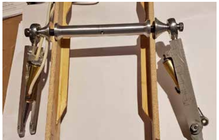
Hank designed/built locking drag links and central reinforcement/pivots with Heim joints
