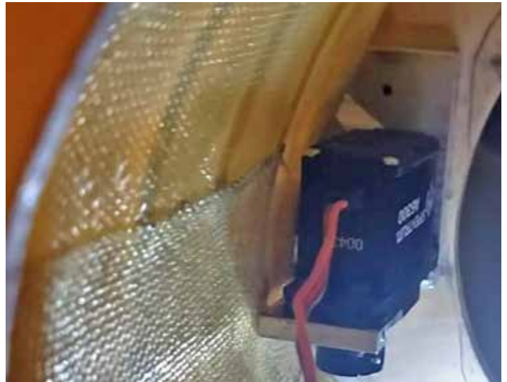
A speedbrake servo on its multi-purpose mount
