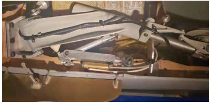
Hank designed/built locking drag links and central reinforcement/pivots with Heim joints
