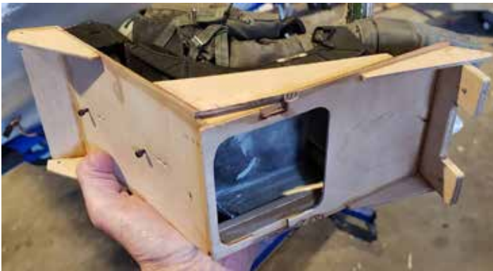
The Airworld cockpit was too flimsy so Hank made replacements out of wood and molded plastic
