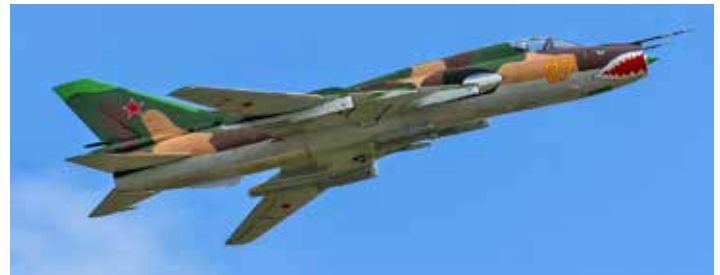
Ron's Su-17 Fitter with the wings swept back to mid position
