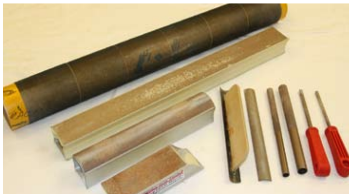
Experiment based on your needs. Note the sanding drum made from a heavy cardboard tube, sanding screen and various straight and curved Permagrafit sanding bars.
