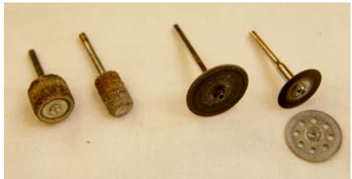
(Left set) Paper sanding drum and a Permagrafit drum. (Right set) To the left is a fiber cut-off wheel and to the right are two version of diamond-coated cut off wheels.
