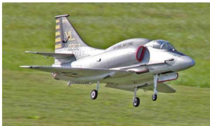
Tam Jets A-4 equipped with the new Jet Cat P-100, making its U.S. debut. The 22.5 pound thrust turbine had no problem powering the 48 inch span jet off the grass runway.
