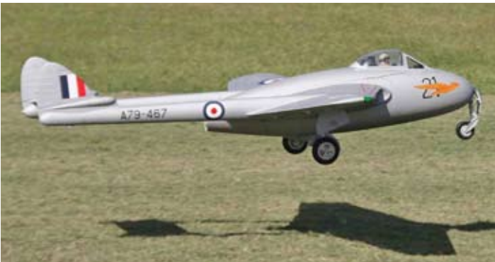
Jim Hiller's de Havilland Vampire completing one of many flights. The 1/5 scale, 30 pound Der Jet model flew nicely with a Jet Central Rhino .
