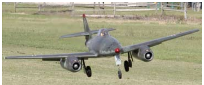
Gun ports and disguised fuselage vents cleverly used as air intakes for the internally mounted turbine. Best Military Jet runner up award.
