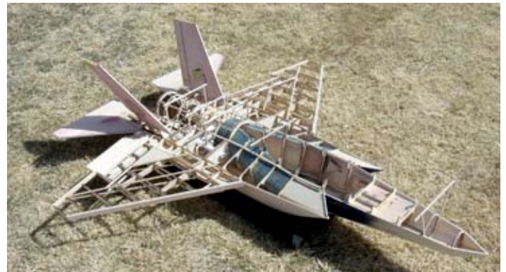
Bob Reynolds’ own design F-35C gets some sun to help the glue dry on the 196 laser cut parts.
