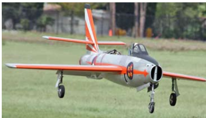
F-84 Thunderjet (sans canopy) on approach. 105" wingspan jet weighed 48lbs and is controlled with a Futaba 14z.
