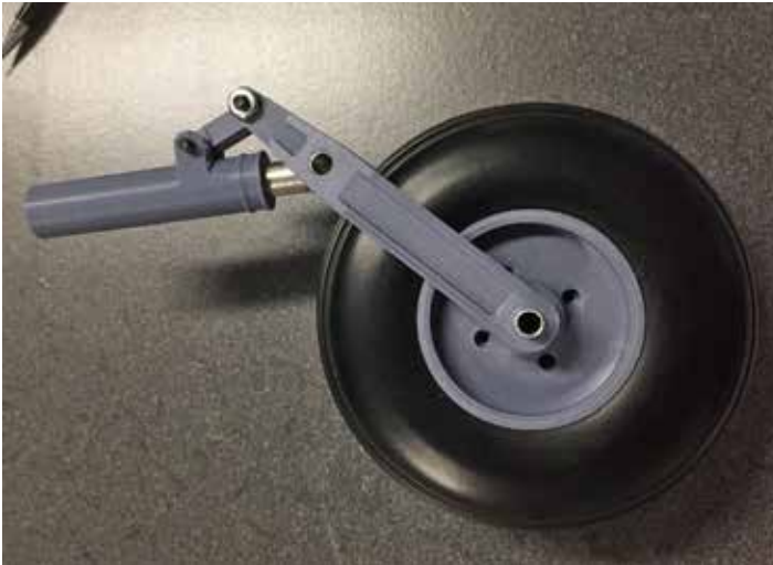
NLG prototype in ABS - above, and a machined set (with extras) - below.
