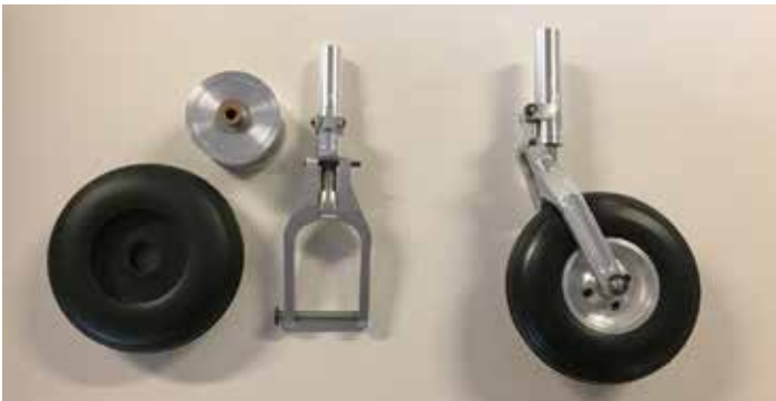
NLG prototype in ABS - above, and a machined set (with extras) - below.
