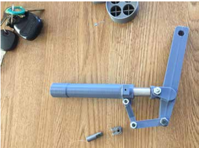
MLG prototype, again in ABS.
