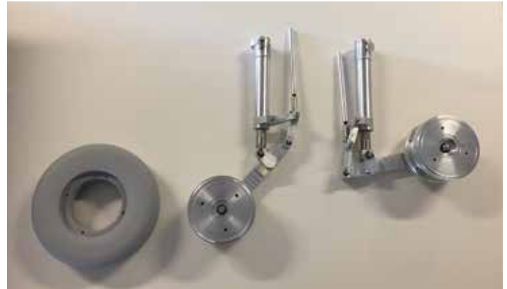
One set (for now) of Machined MLG.
