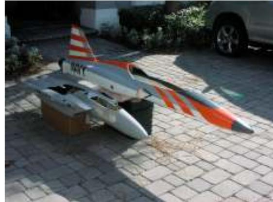
**Weight:** Fuse weight with three 4000 Mah Lithium Ion packs is 24.3 lbs. Wings are identical at just under 5 pounds each, and the cockpit/canopy weighs 2.5 pounds (more on this later). With 12 ounces of lead in the nose to balance, all up weight came in at just over 37 pounds. I think I could have minimally brought the plane in at 35 pounds, but can't see it lighter at the proper CG.
