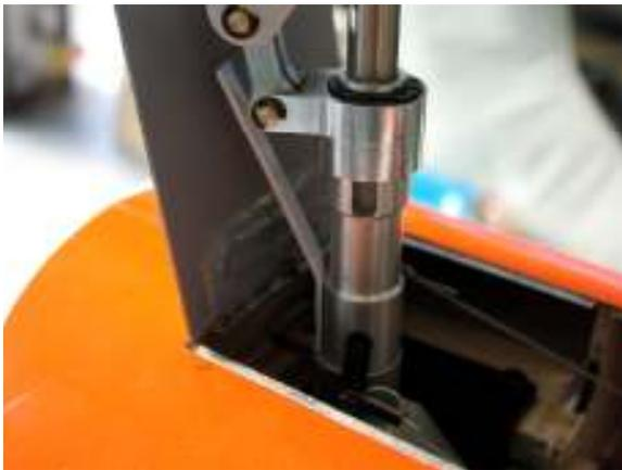
The nose gear does not come with a particularly good mechanism for holding the gear centered when retracted. I solved this problem by gluing small ply blocks to the firewall, positioned such that the steering arms sit on them when the gear is up. This effectively locks the gear in place.
