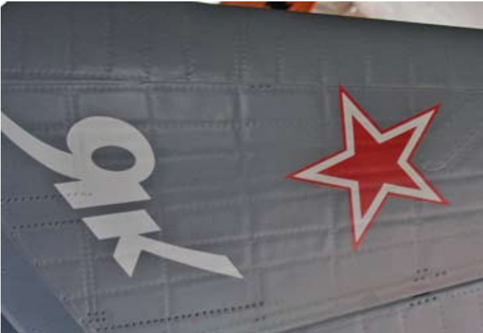
Note the puckered metal around the simulated rivets on the fin of the Yak.
