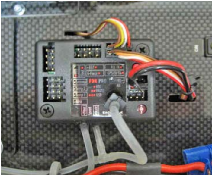
At 2 x 1.4 x 3/4 inches, and weighing only 1 ounce, the data recorder takes up little space. Note that "RPM," "temp," "EGT" and other input slots on the recorder are designed for gas/glow engines and are not usable for turbines.
