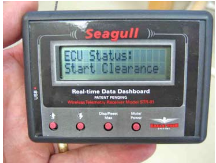
Handheld "dashboard" display unit. Up/down arrow buttons navigate between screen displays. ECU Status screen shown is very convenient for start-up.
