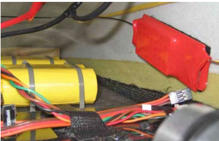
The 1/4 inch thick telemetry transmitter is Velcroed to the fuselage side. A 5-inch wire antenna sticks up into the nose.
