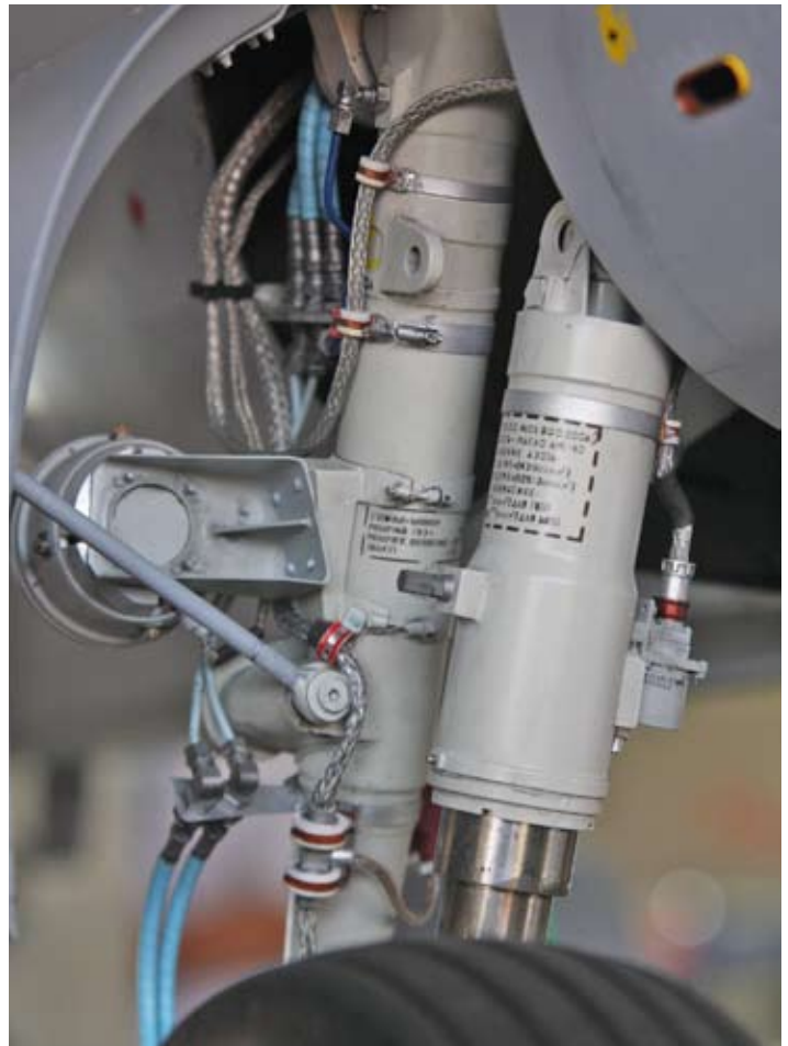
Main gear of the Russian Yak. The gear is high pressure molded carbon. Add in the metal braided cables and accessories and it passes for full scale when just inches away from it.
