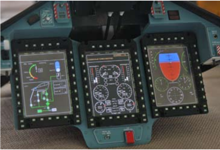
Fully lit up digital glass cockpit screens in the Russian Yak 130.
