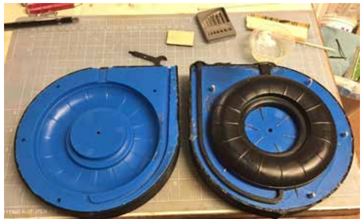
A finished tire ready to remove from the mold.
