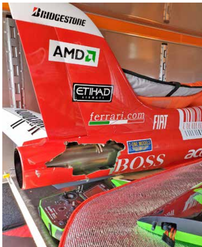
Mike Basso had an inflight H-stab failure on this Viperjet .
