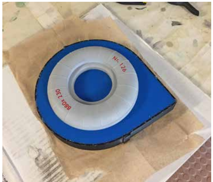
Tire plug with first half of the mold poured.
