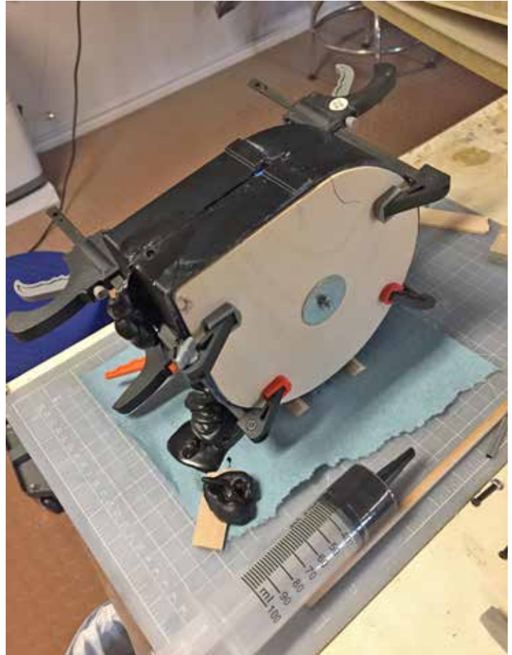
Filling mold with syringe.
