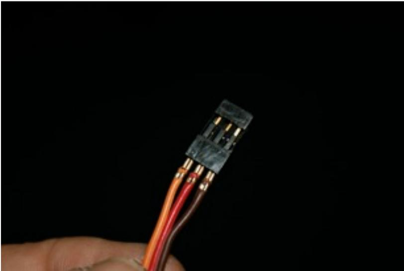
Flip the plastic end over, and using your small screwdriver, push each of the connectors into place until the hold down tab clicks. Don't squeeze these tabs too hard or you will break them off. For some reason, this is
