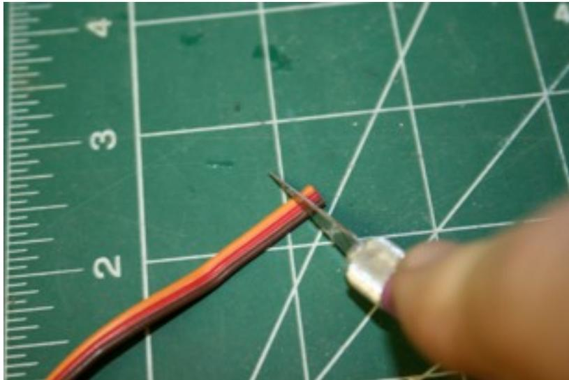
Using your thumbnail, peel away the insulation from the end of the wire. Using the knife, carefully separate the three wires for about .5". You should now have three wires with an identical length of bare wire exposed.
