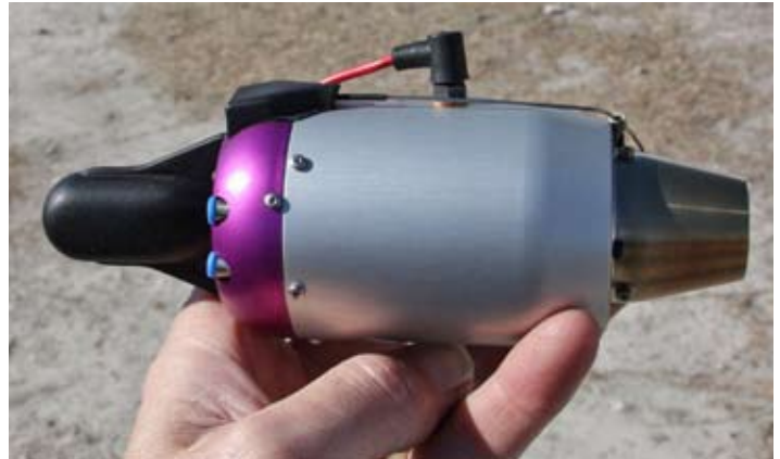
In contrast, tiny JetCat P-20 needs 245,000 rpm to produce 5 pounds of thrust! Only uses 3oz/minute of Jet A in the process.
