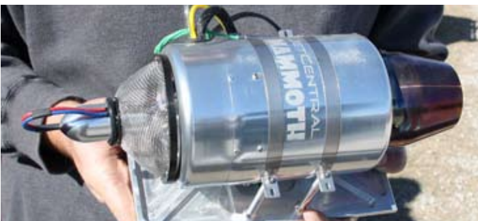
First public viewing of the new Jet Central Mammoth. Impressive specs including 48 pounds of thrust at only 104,000 rpm.
