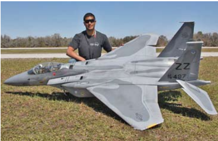
"Centerline" thrust, twin-powered Fei Bao F-15 only needed "a little rudder input" when an engine quit at liftoff according to pilot Adrian Valencia. Once on downwind he said "it flew normally."
